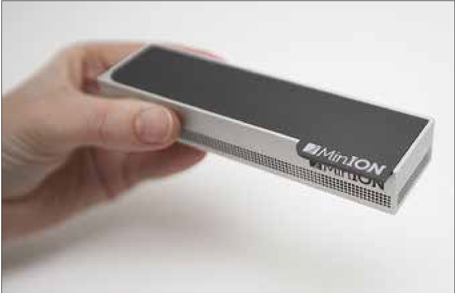
MinION sequencer from Oxford Nanopore Technologies
